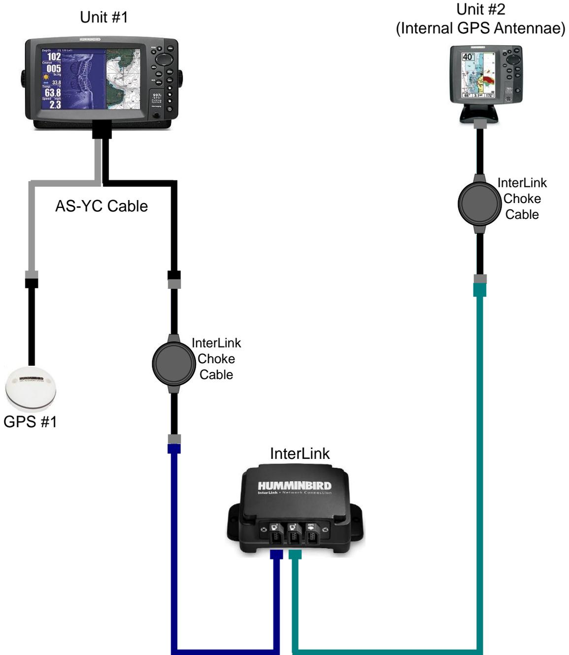
InterLink Choke Cables are only needed if there is electrical interference coming in through the InterLink module.
