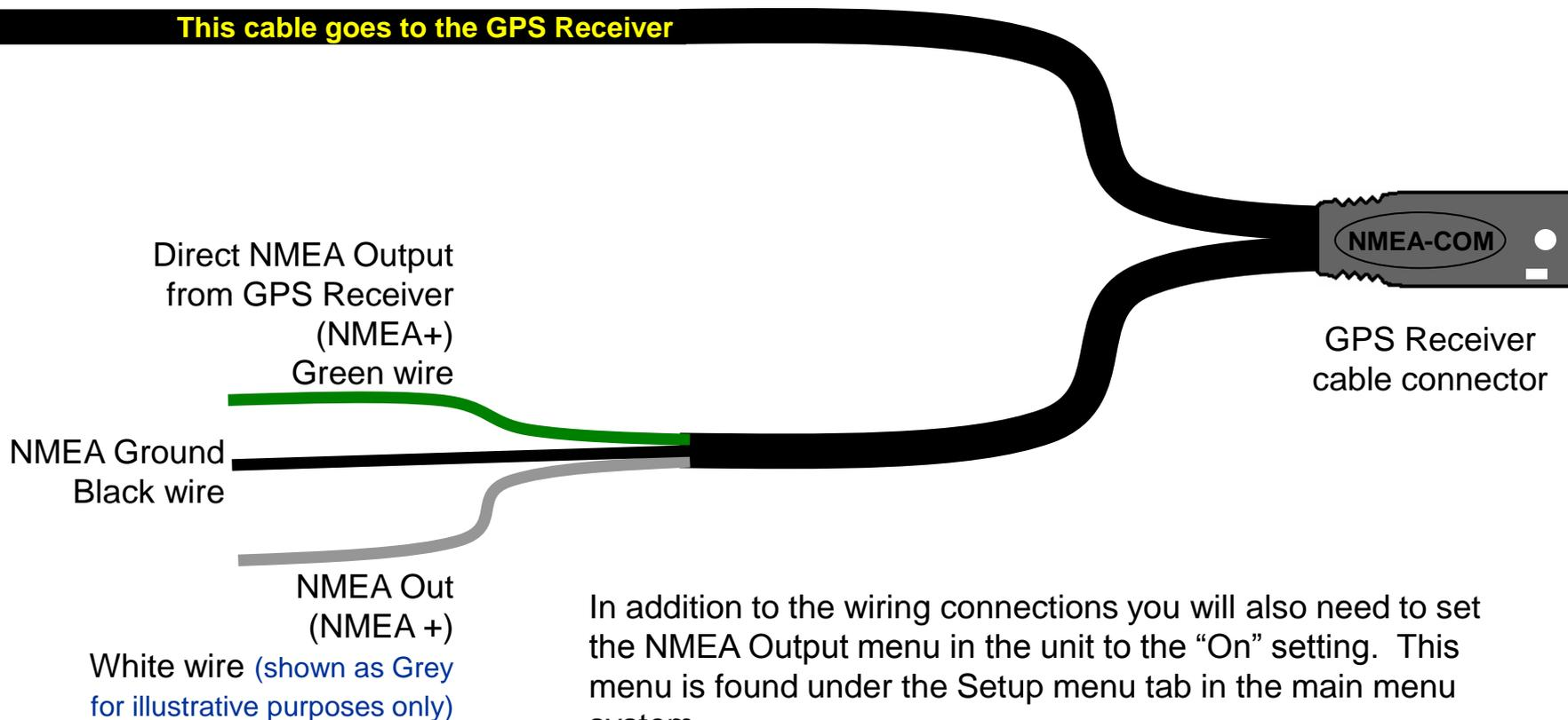
In addition to the wiring connections you will also need to set the NMEA Output menu in the unit to the “On” setting. This menu is found under the Setup menu tab in the main menu system.
