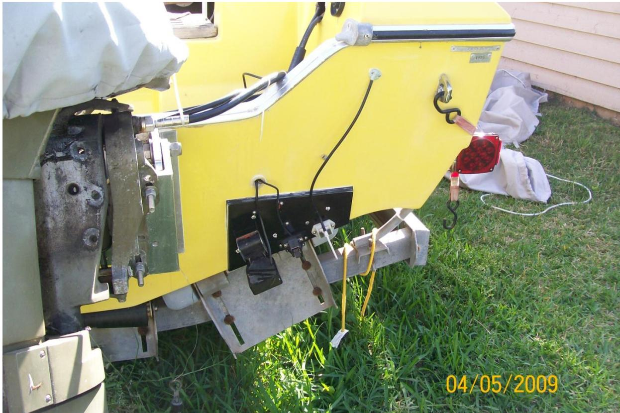
Hard to see since the wires, depth and speed transducers are black like the pad, but hope you get the idea. The stays for the wires and tube are also mounted in the plate.
