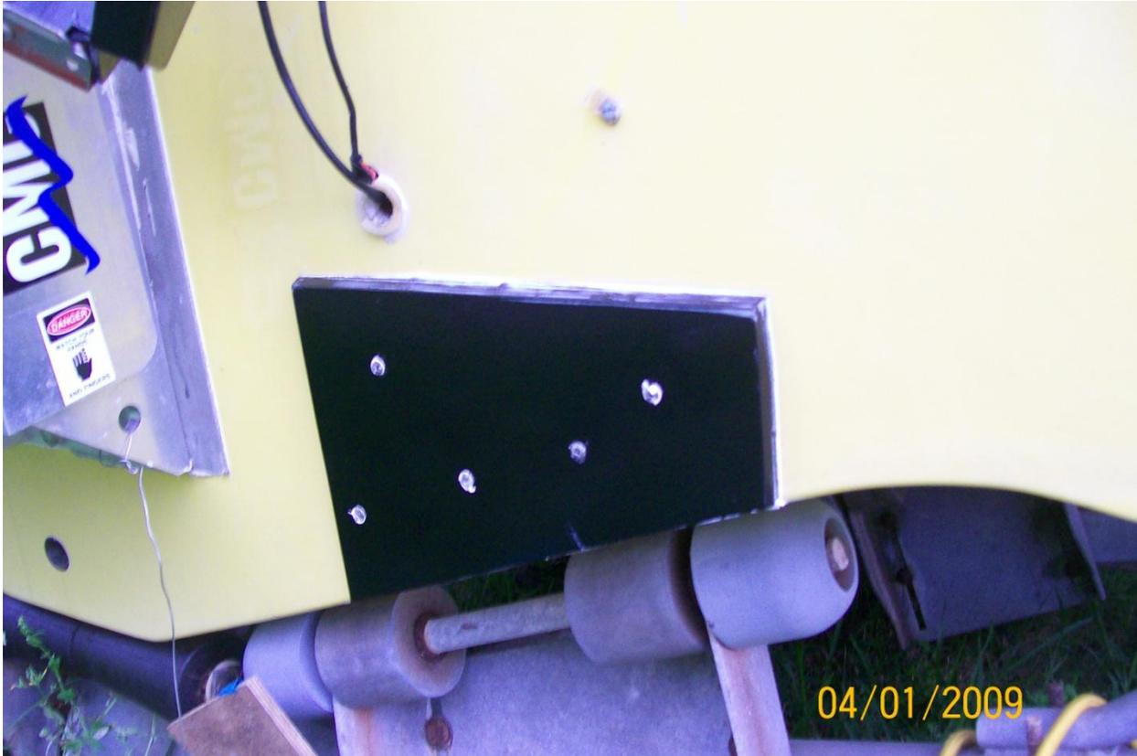
The screw placement is not as random as it looks. The two top screws are aligned horizontal and the three lower ones are parallel with the hull bottom. The idea was to minimize the number of screws used, distribute the forces, and miss possible mounting sites.
