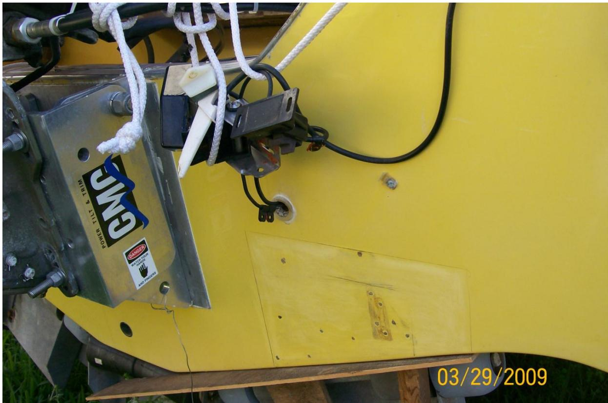
After removing the old mountings, the old holes were drilled out to accept wood dowels that would fit snug. The drilling chips were
