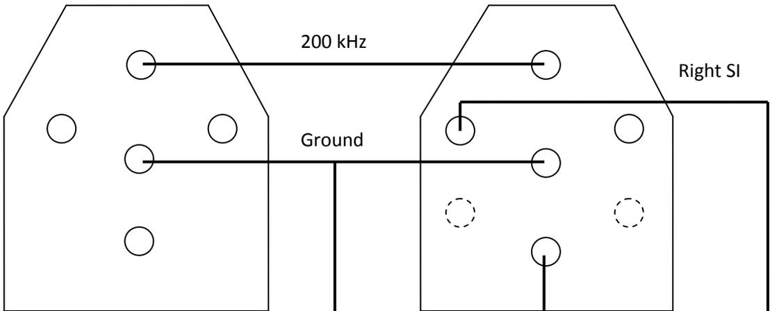
**Wiring between connectors in the LowBird-2 system. Series connection.**
