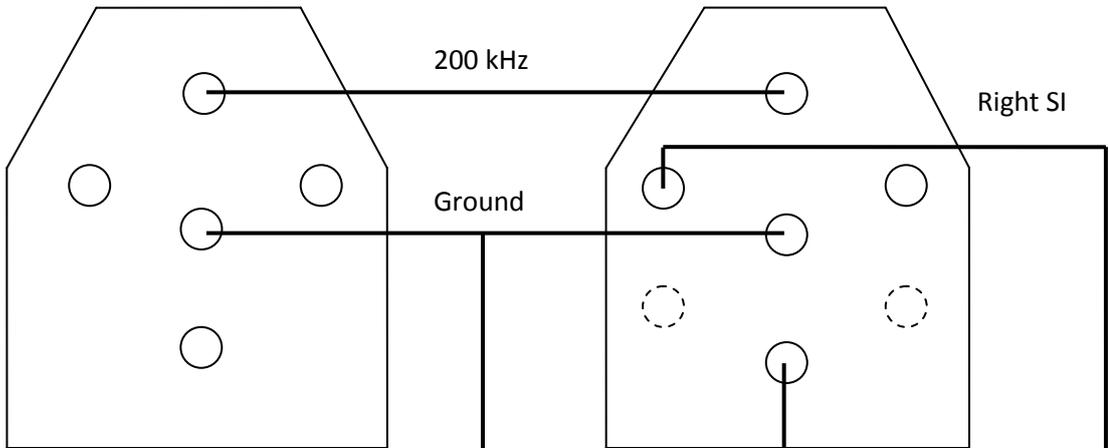
**Wiring between connectors in the LowBird-2 system.**
